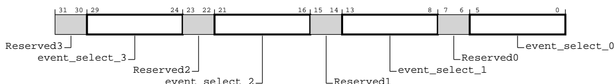
Figure 16-354: Bit assignment diagram for the pmusela register
